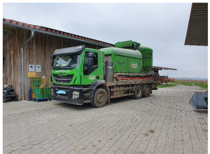
Figure 5: Installation mobile de broyage et mélange. Photo: Christopher Lindner
