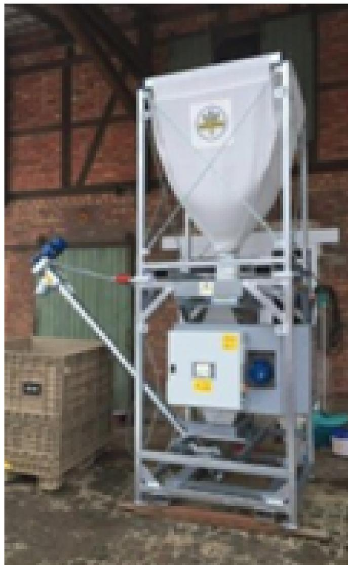
Figura 2: Tostapane mobile - Eco Toast EST GmbH. Fonte: <http://www.sojatoaster.com/referenzen-sicherung>
