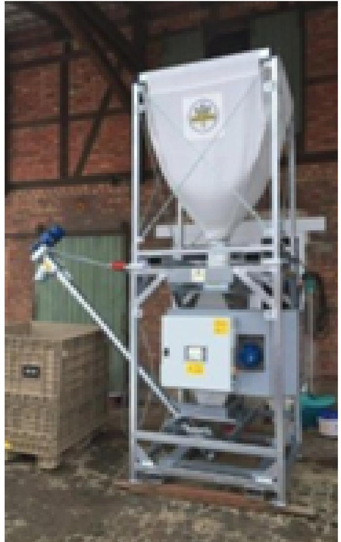
Figure 2: Mobile Toaster - Eco Toast EST GmbH. Source: <http://www.sojatoaster.com/referenzen-sicherung>
