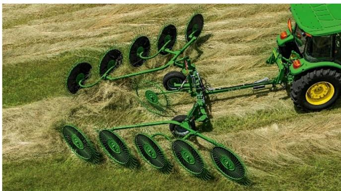
Figure 1: Rowing hay with a tedder. Photo courtesy of John Deere
